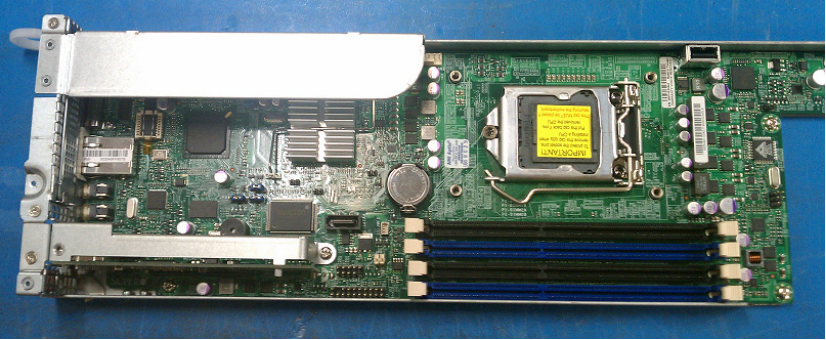
The image above shows the X9SCD-F mounted on a motherboard tray, ready to be inserted into a Supermicro CSE-938H-R1620B 3U chassis.
