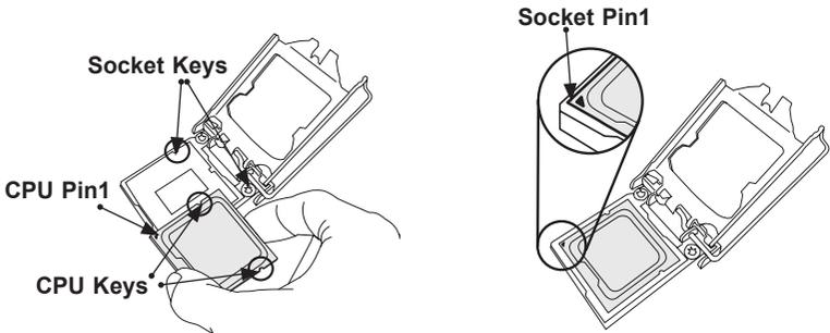
3. Once they are aligned, carefully lower the CPU straight down into the socket. (To avoid damaging the CPU or the socket, do not drop the CPU on the socket. Do not rub the CPU against the surface or against any pins of the socket.)
