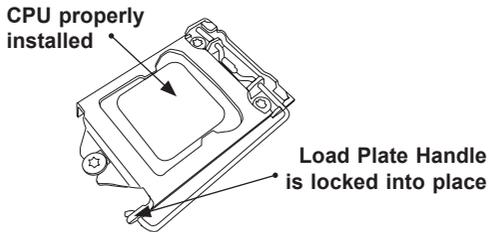
6. When the CPU is securely locked into the CPU socket, the plastic cap will be automatically loosened from the load plate. Use your thumb and index finger to remove the plastic cap from the socket.
