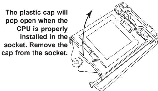
**Warning:** You can install the CPU inside the socket only in one direction. Make sure that it is properly inserted into the CPU socket before closing the load plate. If it doesn't close properly, do not force it, as that may damage your CPU. Instead, open the load plate again and check whether the CPU is properly aligned and securely seated inside the socket.
