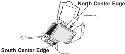
2. Align the CPU keys, which are the semicircular cutouts on the sides of the CPU (shown below), against the socket keys, the semicircular notches on the sides of the CPU socket. Align CPU Pin 1, the triangle at the bottom left of the CPU, against Pin 1 of the socket, the triangle marker at the bottom left of the CPU socket.
