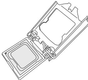
5. Once the CPU is properly installed, use your thumb to gently push the load plate handle down to the handle lock and lock it.
