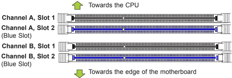
The X10SLD-F/-HF supports up to 32GB of Unbuffered (UDIMM) DDR3 ECC 1600/1333/1066 MHz in 4 memory slots. Populating these DIMM modules with a pair of memory modules of the same type and same size will result in interleaved memory, which will improve memory performance. Please refer to the table below:
