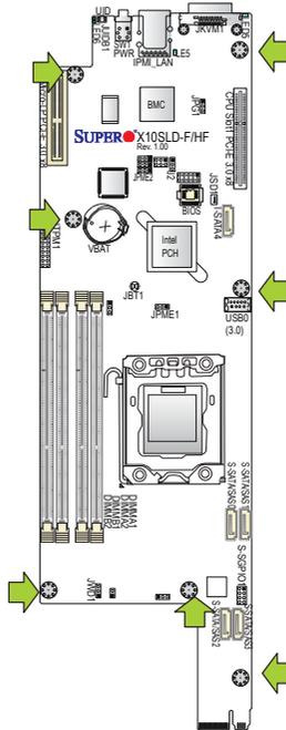
**Caution:** 1) To avoid damaging the motherboard and its components, please do not use a force greater than 8 lb/inch on each mounting screw during motherboard installation. 2) Some components are very close to the mounting holes. Please take precautionary measures to avoid damaging these components when installing the motherboard to the chassis.
